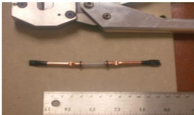
Figure 1. Passive diffusion sampler used for collection of dissolved noble gases in water samples.
